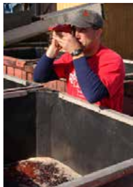
Winemaker tests for Brix with a refractometer.
