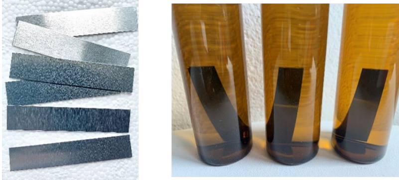
Figure 1 - (left) Aluminum coupons coated with common can coating materials; (right) coated coupon immersed in white wines for accelerated aging trials
