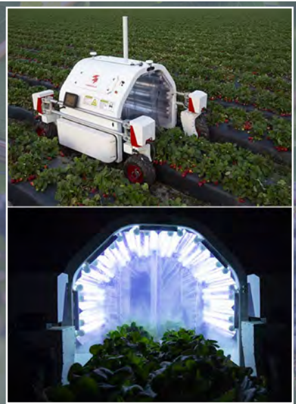
Figure 4. Thorvald, an autonomous robotic device developed in collaboration with SAGA Robotics in Norway, can carry and power the same UV array used in tractor drawn devices.
