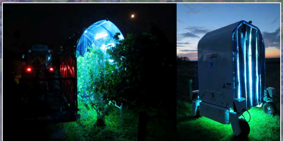
Figure 9. A tractor-drawn UVC lamp array used to treat grapevines at Cornell Agritech, and the same array carried by the autonomous robot Thorvald, manufactured by Saga Robotics.
