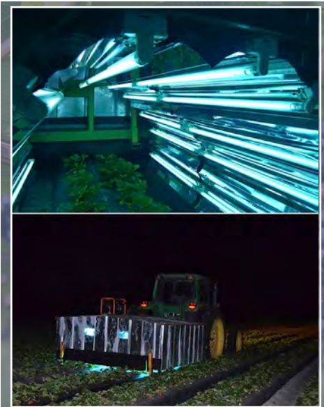
Figure 3. Tractor-drawn UVC array used in the first large-scale field trials on strawberries. Side-by-side arrays allowed two rows to be treated in each pass.
