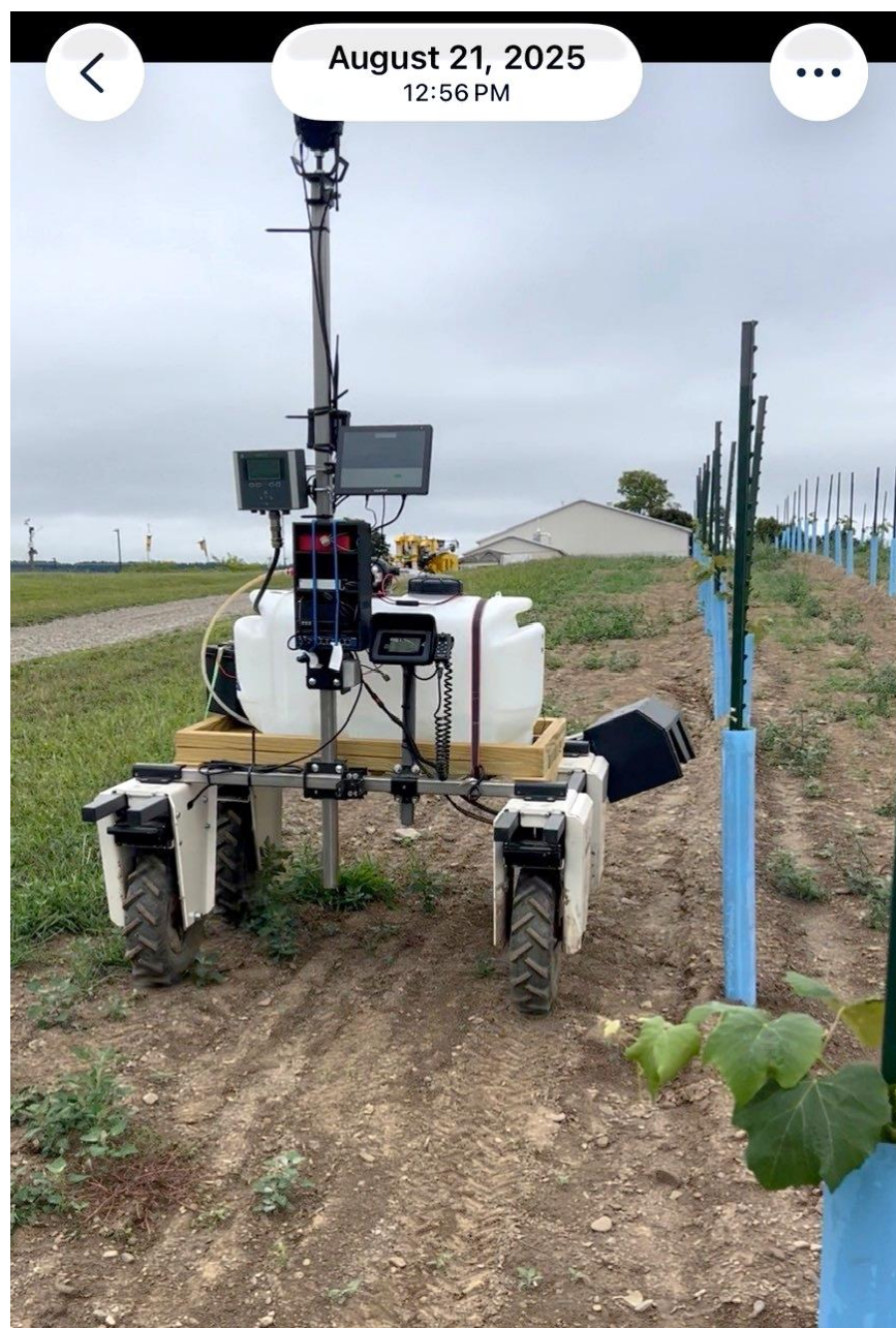
Figure 1. Cornell's autonomous Bonsai Amiga - Weed-IT™ spray system operating in a newly planted vineyard (2025) located at CLEREL in Portland, NY.
